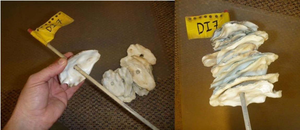
Figure 3. Shell-string collector assembly.
