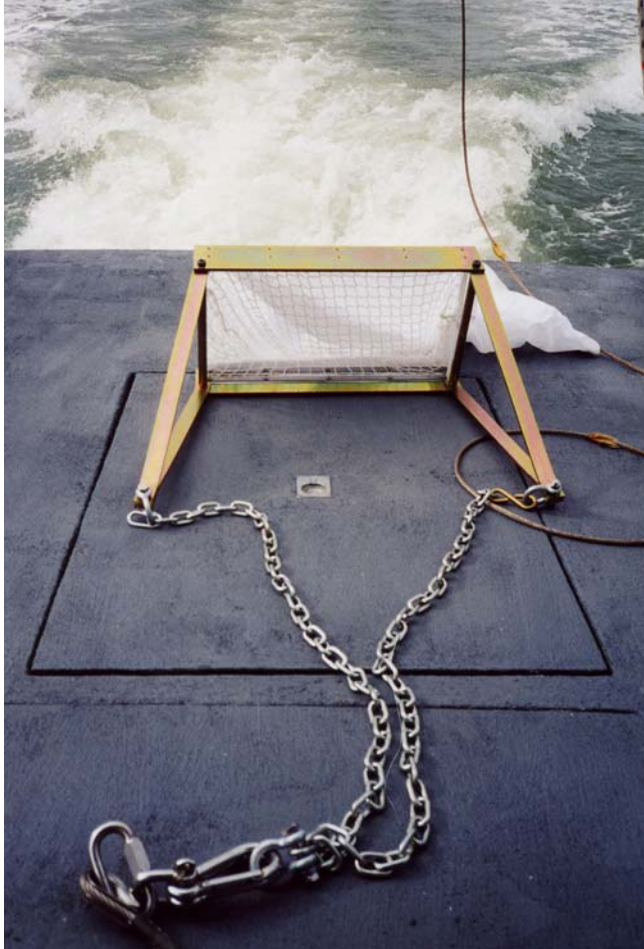
Figure 2. Wildco biological oyster dredge, (50-cm mouth, 2cm mesh) on the stern of the RV Questuary, October 4th, 2001. Cable is hooked up to hydraulic winch. Dredge used for subtidal sampling study.
