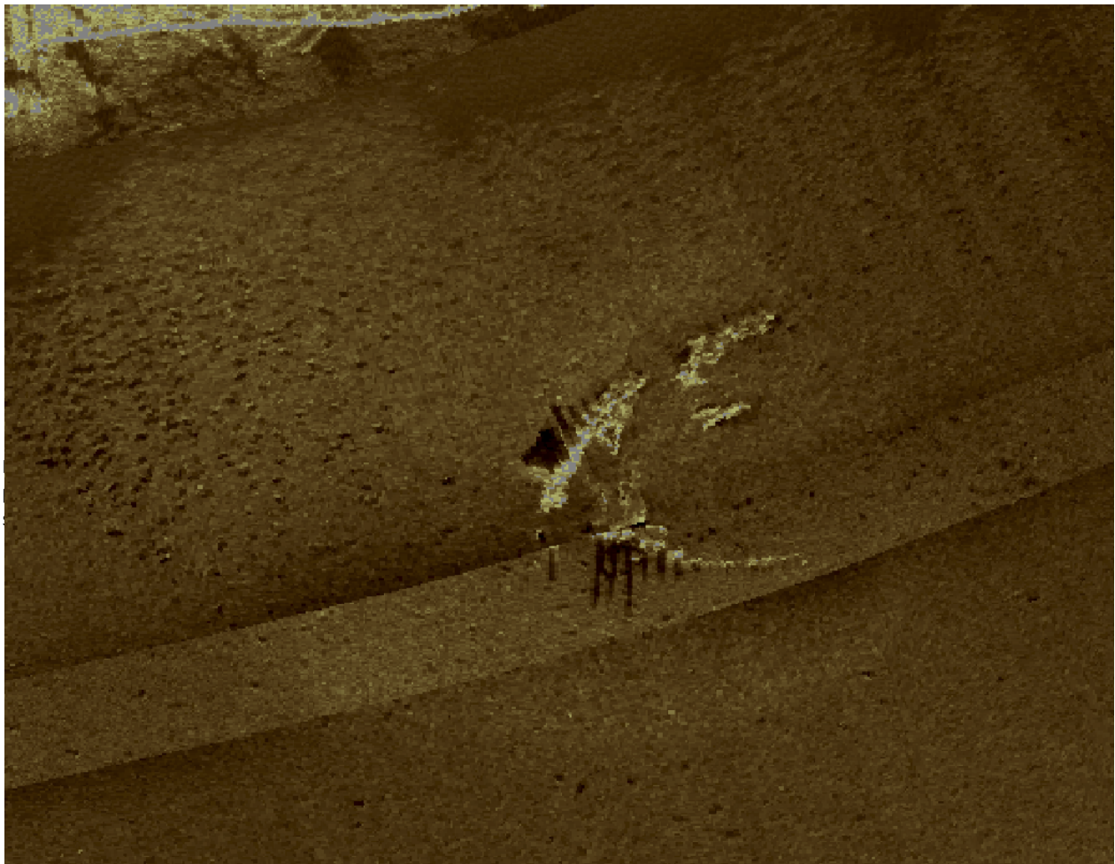
Interferometric sidescan sonar image of ship ribs at bow emerging from the bottom within a scour hole generated where the piling wall of the ferry pier has been breached. The vessel is a minimum of 4 feet below the sediment surface and may have been buried in the sediment prior to pier construction.
